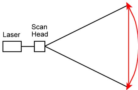
Angular Velocity is the speed that the beam moves times the angle of scan
