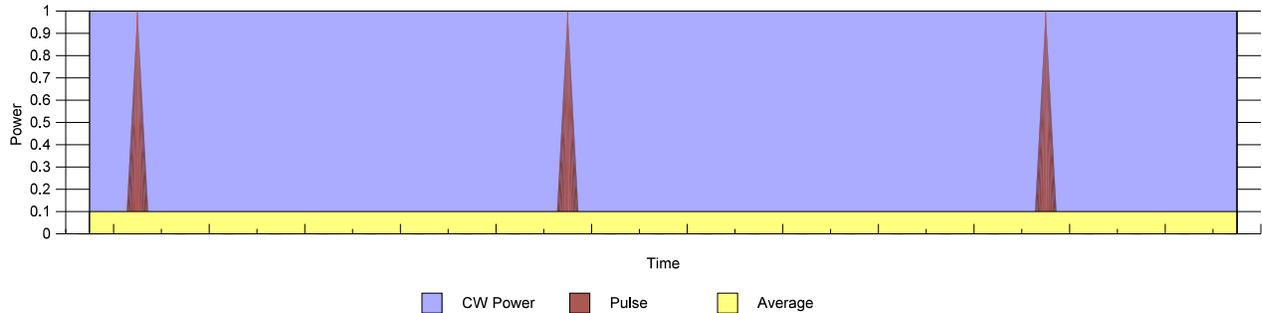
To find the radiant exposure for a single pulse, we take 1.27 W/cm<sup>2</sup> times the 10 microseconds of exposure, and arrive at 12.7 microjoules/cm<sup>2</sup>. 100 successive pulses (a second's worth of energy) adds to a total of 1.27 millijoules/cm<sup>2</sup>. This is also equivalent to an average irradiance of 1.27 milliwatts/cm<sup>2</sup>.
