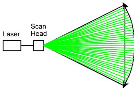
Energy at one location can be reduced by scanning, where the power is “spread out” over the scan path
