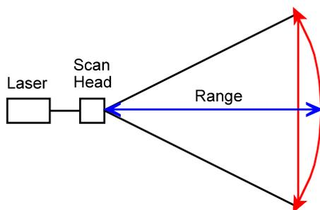
Linear Velocity is Angular Velocity times Range, and is the rate that the beam moves past a specific location at that range
