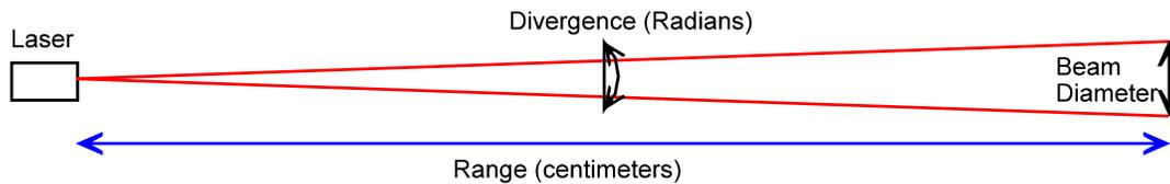
Beam Diameter at a distance is the divergence of the beam times the range
